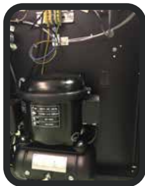
Silent compressor inside the machine
